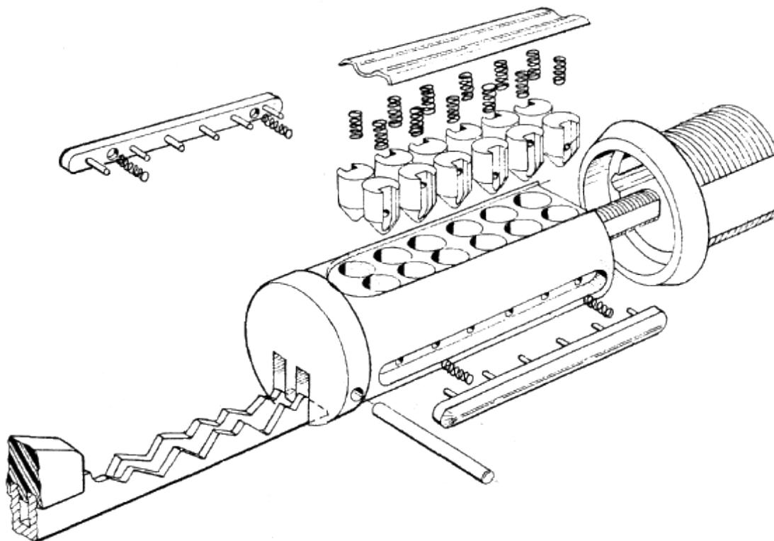
**Figure 1.1:** Cylinder design from the BiLock First Generation patent (US 4,478,061)
