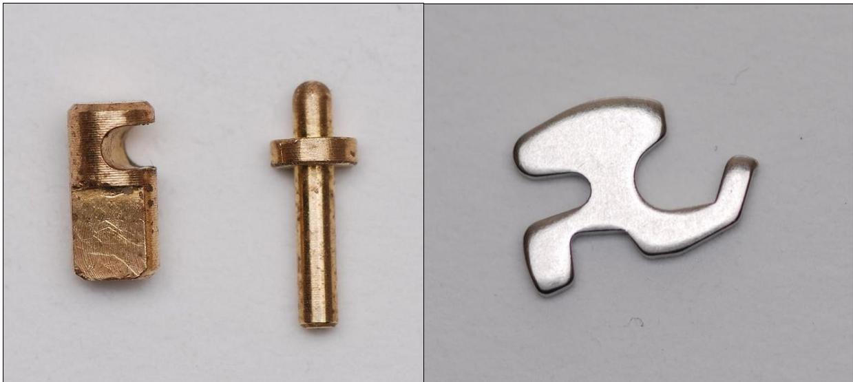
**Figure 2.3:** The plug's two NG components (left) and the key's moving element (right).
