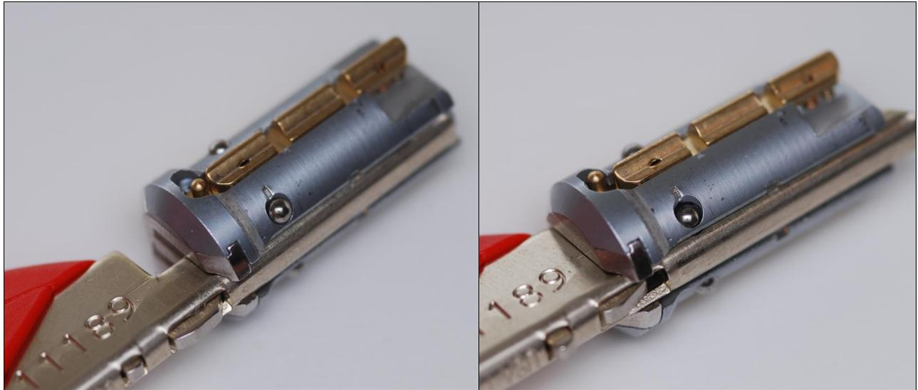
**Figure 3.3:** Control key bearings in the locked (left) and unlocked (right) positions.
