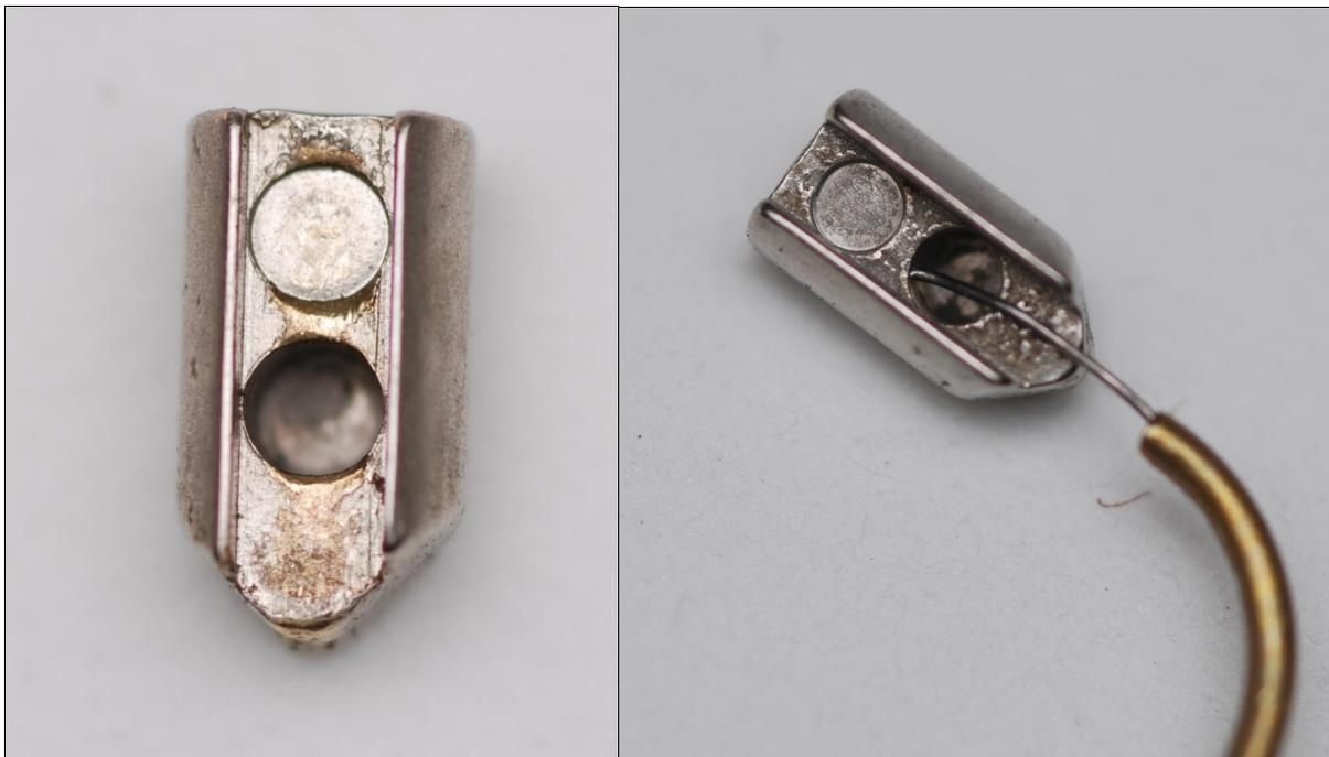
**Figure 4.3** (Left): The channels on each pin extend through the length of the pin.
