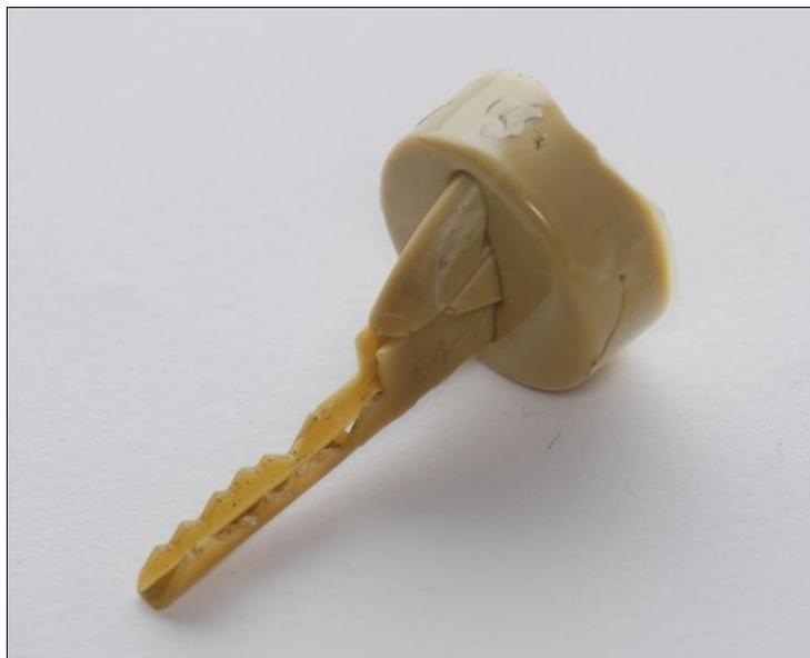
**Figure 4.2:** A BiLock NG key molded with silicone and cast using urethane.
