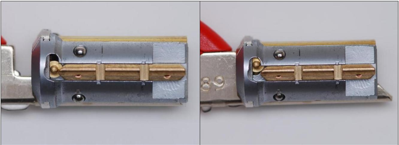
**Figure 2.5:** The moving element in the lowered (left) and raised positions.
