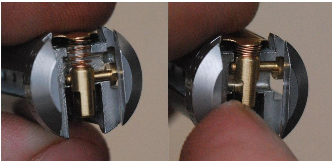
**Figure 2.4:** The plug's NG component is moved to free the right hand sidebar.
