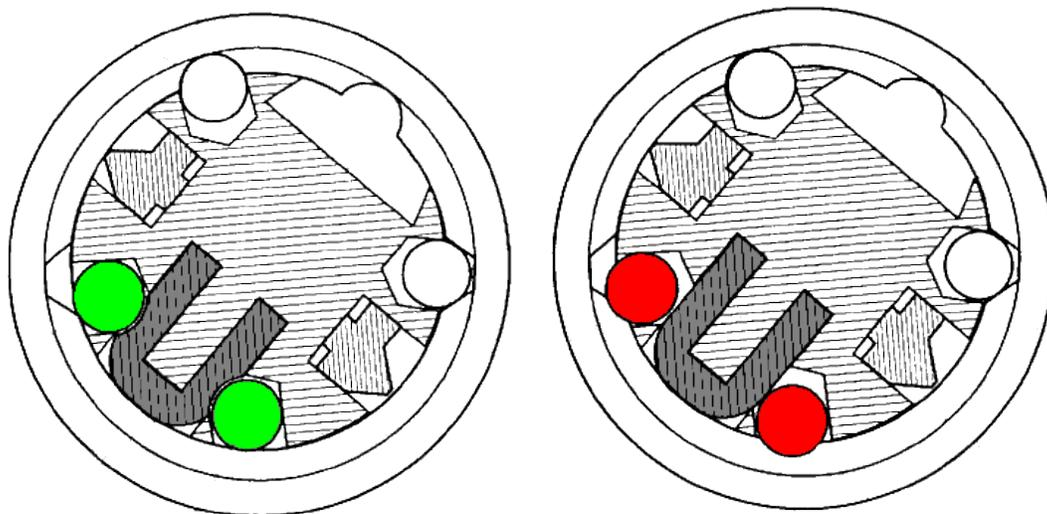
**Figure 3.2:** Control key (colored) and retainer bearings (white) in the plug. (US 6,076,386)
