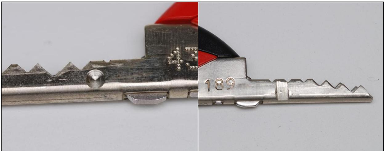
**Figure 3.4:** A QC control key (left) and modified user key (right) that can remove cores.
