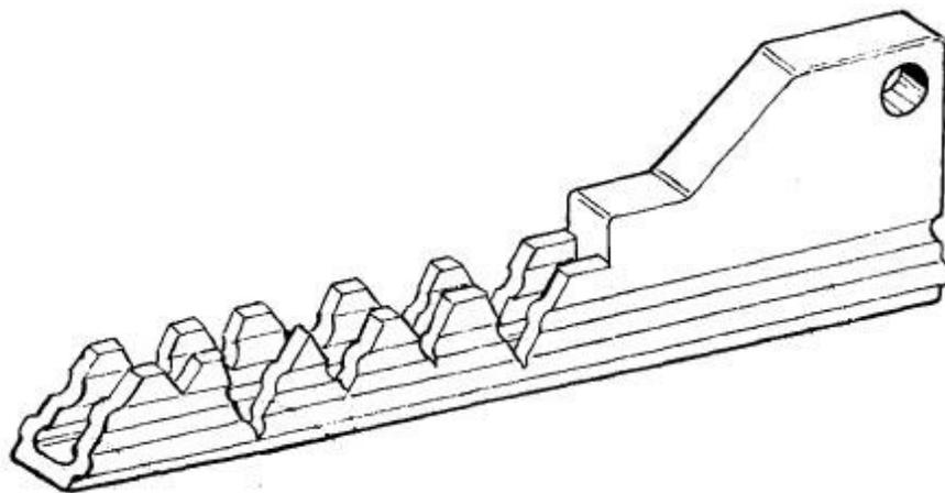
**Figure 1.8:** Key warding example from the BiLock First Generation patent (US 4,478,061)
