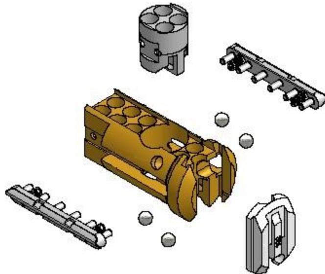
**Figure 5.1:** New BiLock design (QC) with steel sidebars and anti-drilling plug modification.
