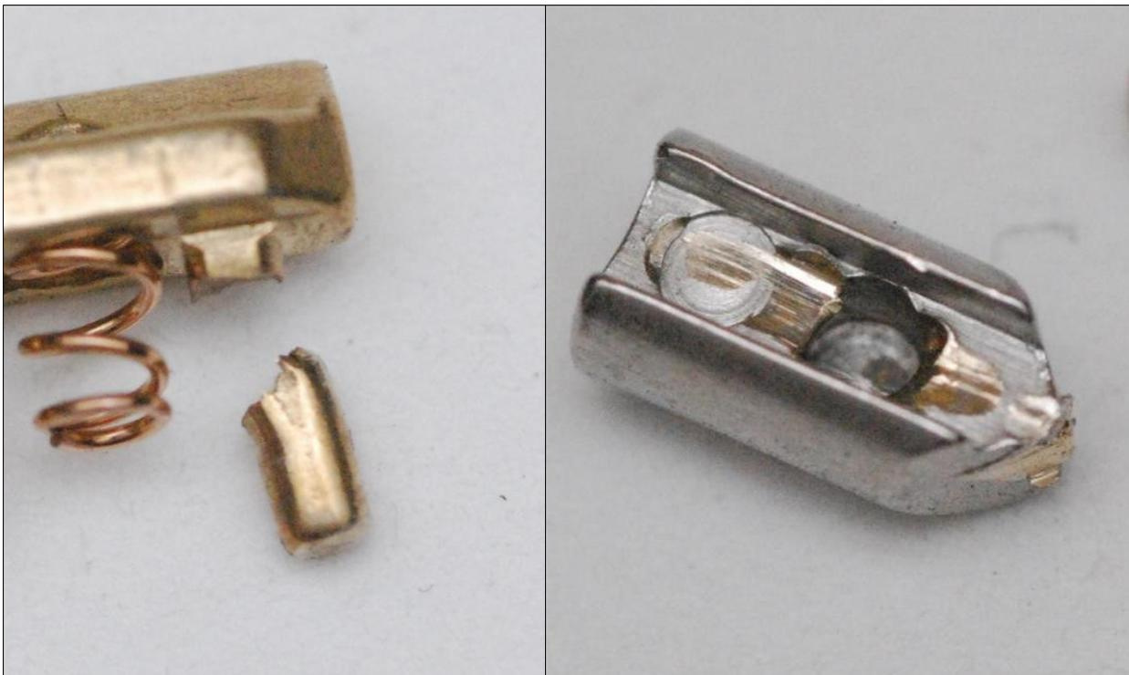
**Figure 4.7** (Left): Sidebar legs can be sheared via torque and vertical movement of the pins.
