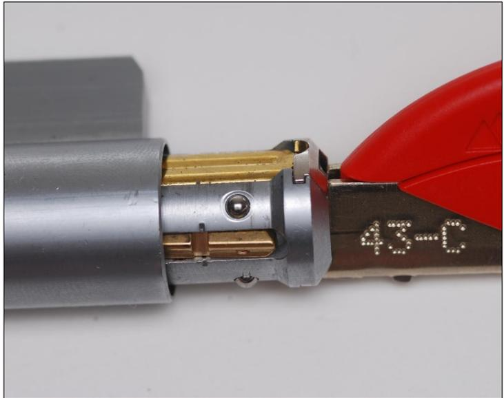
**Figure 3.1:** The BiLock QC core being extracted.
