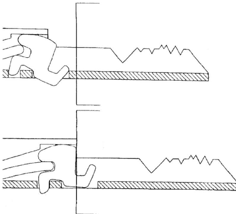
**Figure 2.2:** The key's NG component is rotated into position by the plug face. (US 6,681,609)
