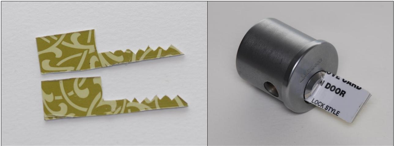
**Figure 4.1:** BiLock keys made out of magnetic stripe cards opening a BiLock rim cylinder.
